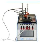
Fluids are equipped with adjustable holders support the probes under test or thermometers
