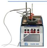
Fluids are equipped with adjustable holders support the probes under test or thermometers
