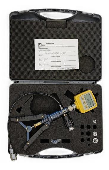
The **LPP 60** hand-held calibration test pump is used for pressure generation for the verification, adjustment and calibration of mechanical and electronic pressure measuring instruments by comparative measurement. These pressure tests can be carried out on the move, on site at the measuring point, or stationary in the laboratory or workshop.
