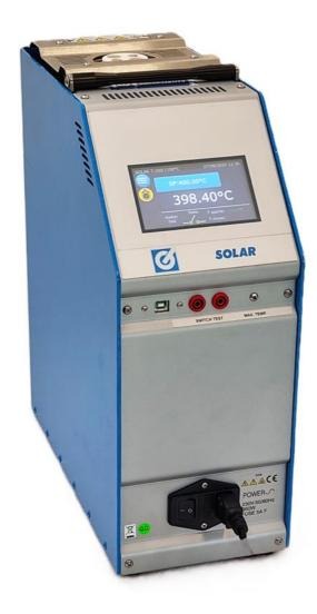
The new **SOLAR T** are portable thermostatic calibrators for laboratory and field testing of temperature, thermocouples and Pt 100 sensors. They consist of a tubolar vertical well with an internal ceramic element to isolate electrical parts and an interchangeable equalising block.
